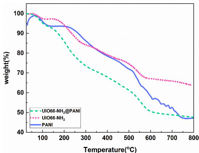
Figure 4 : TGA thermogram of the UIO66-NH<sub>2</sub>, PANI and UIO66-NH<sub>2</sub>@PANI
