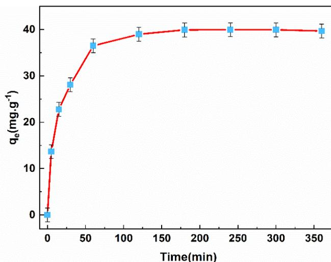
Figure 5 : Adsorption kinetic profile of UIO66-NH<sub>2</sub>@PANI nanocomposite
