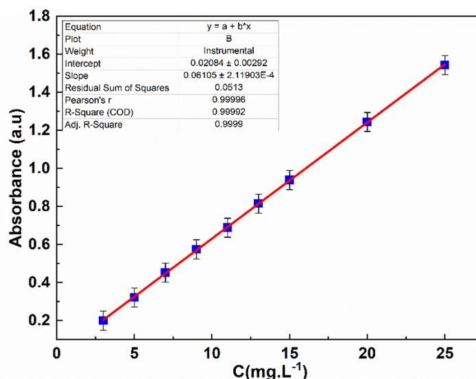
Figure 2 : Calibration Quercetin (3-25 mg/L)
