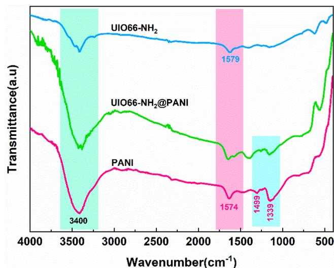
Figure 3 : FT-IR spectra of the UIO66-NH<sub>2</sub>, PANI and UIO66-NH<sub>2</sub>@PANI
