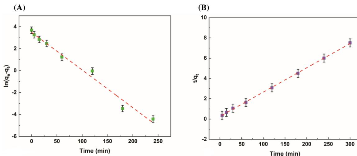
Figure 6 : Plots of kinetics model P.F.O (A), P.S.O (B)
